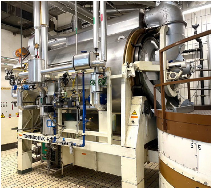
The moisture is removed from the cocoa nibs in the large roasting drum. Right: The three KMA gas scrubbers cool, humidify and clean the cocoa exhaust air in preparation for the biofilter.
