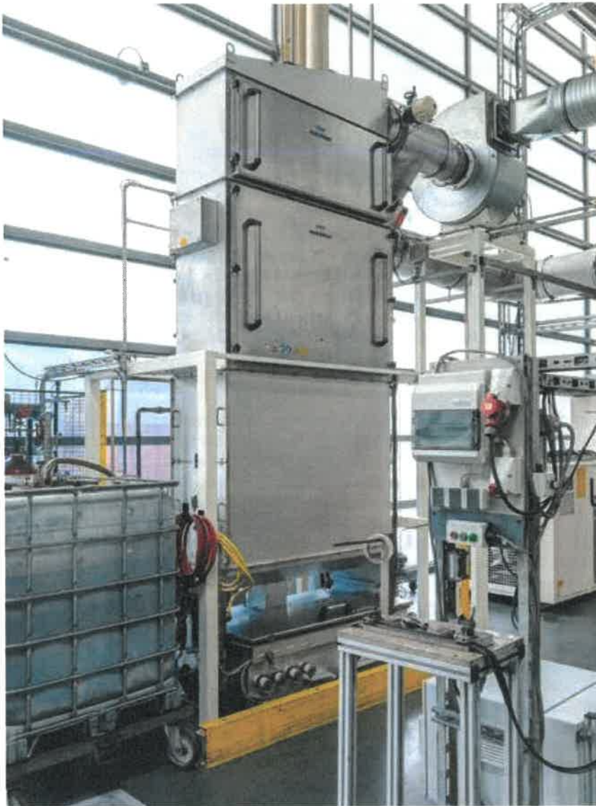
The individual modules for exhaust air purification are arranged one above the other and thus require little floor space.
